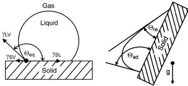
**Figure 1:** Static and dynamic contact angles over a surface. [2]
