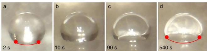
**Figure 2:** Structural transformation of the droplet on a superhydrophobic surface while cooling from room temperature to  $-10^\circ\text{C}$ .
