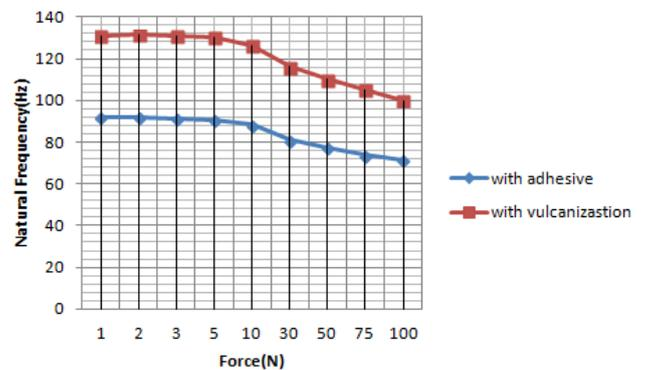
Fig. 3. Natural Frequencies based on Loads
