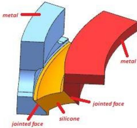
Fig. 1 3 D model of jointed assembly
