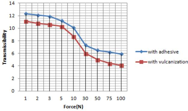
Fig. 4. Transmissibilities based on Loads
