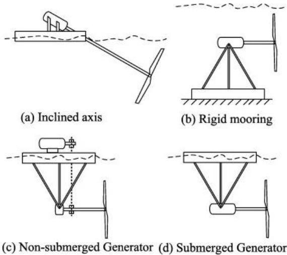
Fig. 1 Horizontal axis turbines [5]
