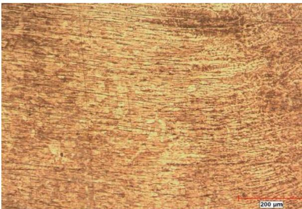
Figure 5. Microstructure image obtained in 70 A welding current
