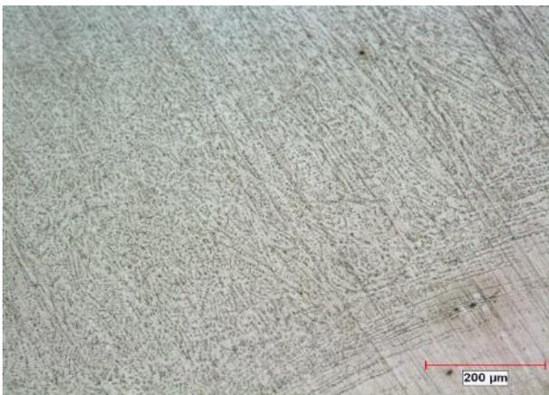
Figure 10. Microstructure image obtained in 110 A welding current in TIG P method
