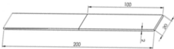
Fig. 2. Measurements of tensile test specimens
