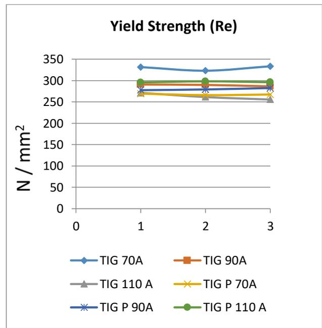
Figure 4. Yield Strengths of welded specimens
