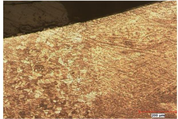
Figure 6. Microstructure image obtained in 90 A welding current
