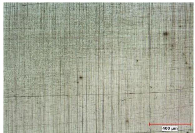
Figure 8. Microstructure image obtained in 70 A welding current in TIG P method
