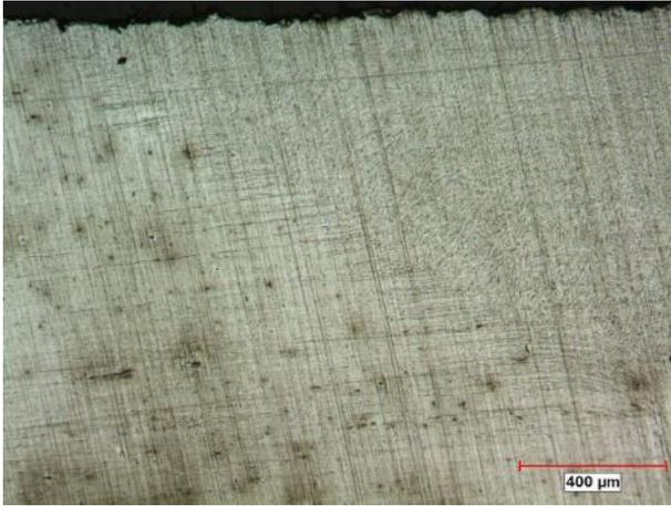
Figure 9. Microstructure image obtained in 90 A welding current in TIG P method
