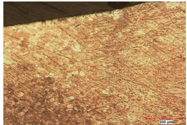
Figure 7. Microstructure image obtained in 90 A welding current
