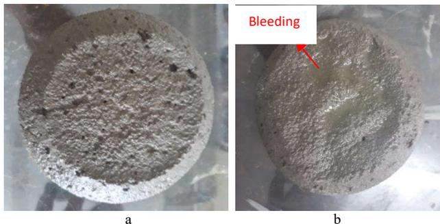
Fig. 4. a) 0.75SPA mortar (Stable), b) 0.75HPA mortar (Unstable and bleeding of mixture due to high HPA dosage)
