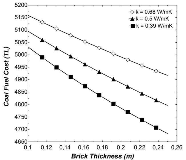
Fig. 3. Change in coal fuel cost due to brick thickness
