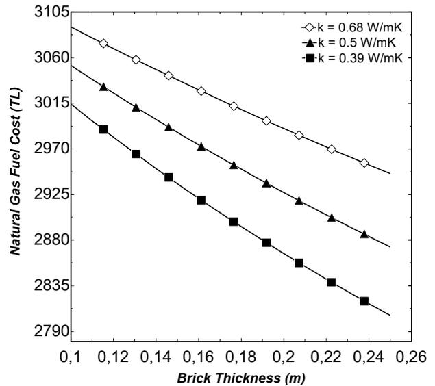
Fig. 2. Change in natural gas fuel cost due to brick thickness
