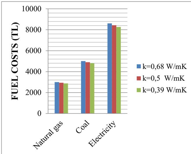
Fig. 5. Change in natural gas, coal and electricity fuel cost due to brick thickness
