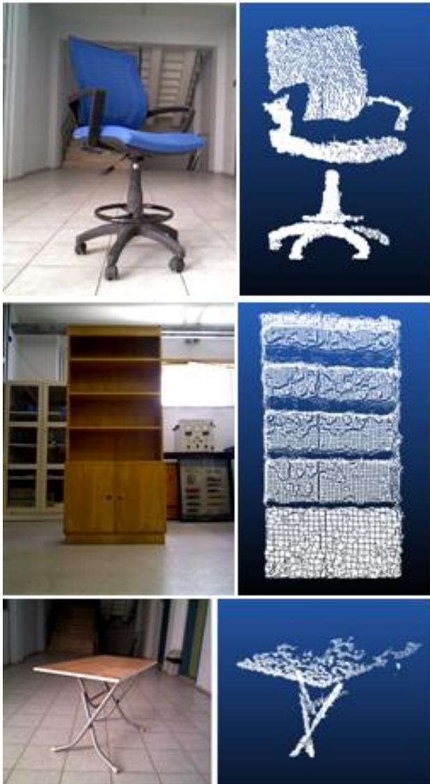
Fig. 9 RGB images (left) and point cloud data examples (right) for chair, bookshelf and table objects captured from real environment
