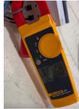
Figure 4 Current measurement during the test
