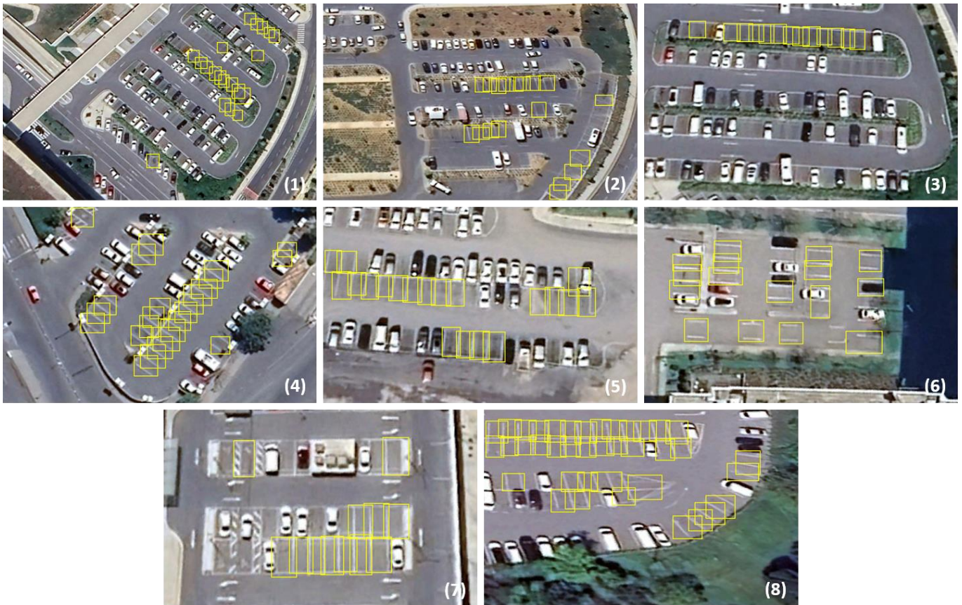
Fig. 2. Examples of vacant parking space detection using the SSD algorithm in various scenarios.
