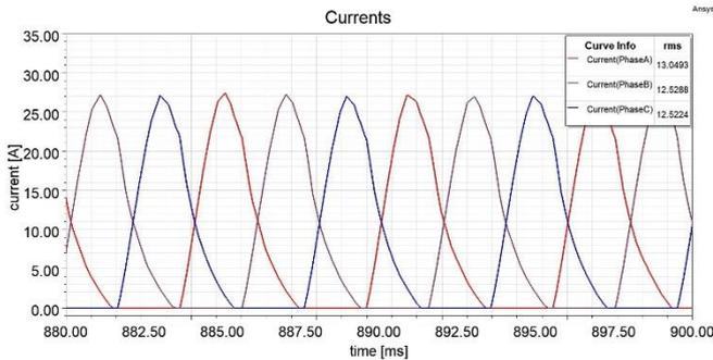
Figure 5 Traditional skewed (5°) rotor SRM currents graphs
