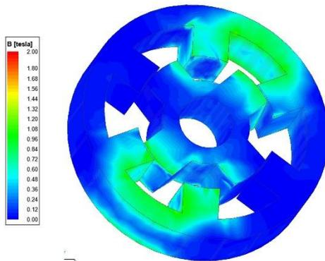
Figure 13 Traditional rotor Skew ( $5^\circ$ ) magnetic flux distribution
