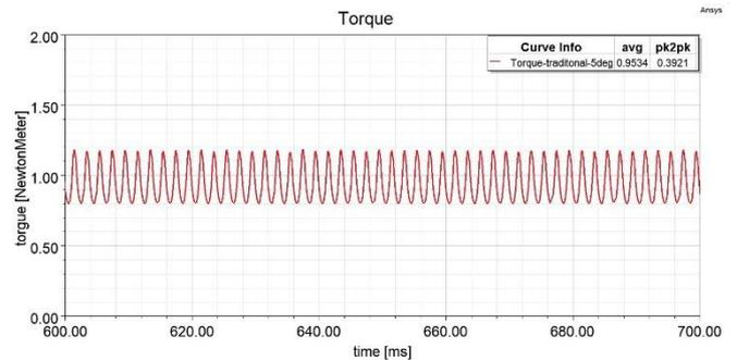
Figure 9 Traditional rotor Skew (5°) torque graphs
