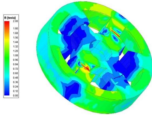
Figure 14 Suggested rotor Skew ( $5^\circ$ ) magnetic flux distribution
