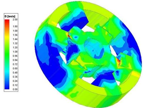
Figure 15 Suggested rotor Skew ( $10^\circ$ ) magnetic flux distribution
