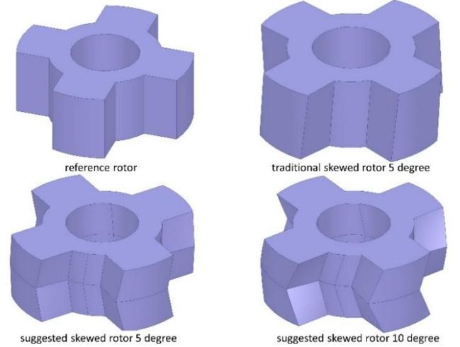
Figure 2 Rotor topologies
