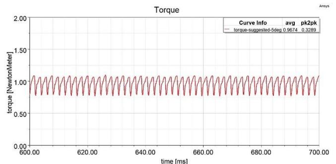
Figure 10 Suggested rotor Skew (5°) torque graphs
