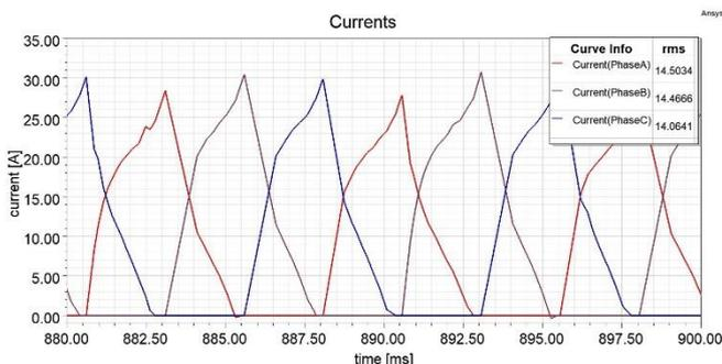
Figure 7 Suggested skewed (10°) rotor SRM currents graphs
