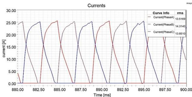
Figure 6 Suggested skewed (5°) rotor SRM currents graphs
