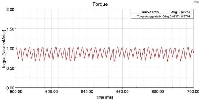
Figure 11 Suggested rotor Skew ( $10^\circ$ ) torque graphs
