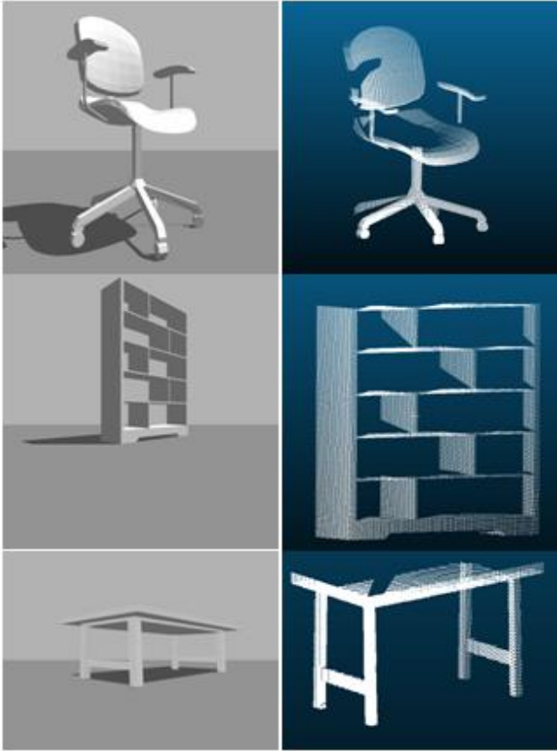
Fig. 7 RGB images (left) and point cloud data examples (right) for chair, bookshelf and table objects captured from Gazebo simulation environment
