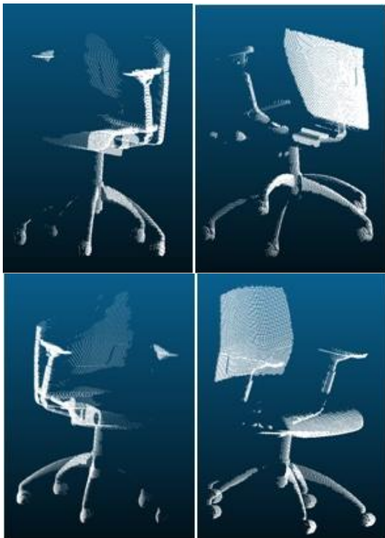
Fig. 4 Point cloud data of a chair taken from 0^\circ , 90^\circ , 180^\circ , 270^\circ angles in Blender simulation environment.
