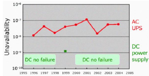
Fig. 2 Data on the reliability of power systems for 23,000 DC and 10,000 UPS systems (NTT Facilities)
