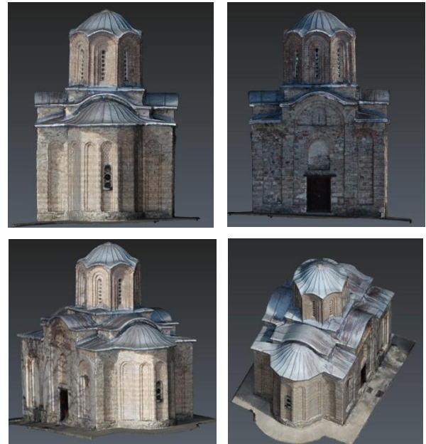
Fig. 3 Generated 3D model of St. Nikita church
