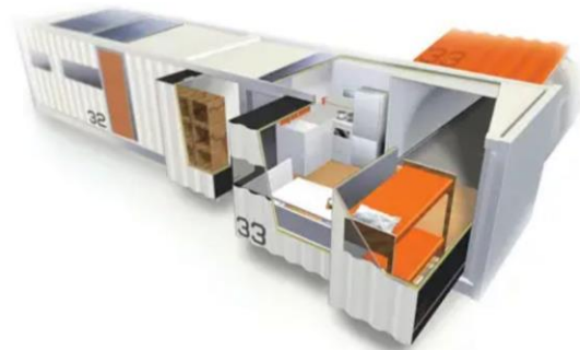
Fig10: example of TED (Transportable Emergency Dwelling) [19]
